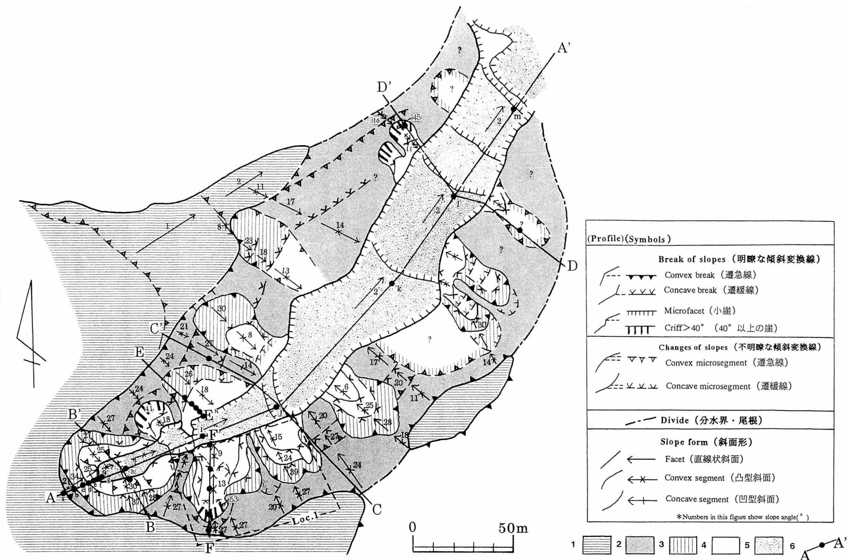
Fig. 6. A morphological map of the study area. 1, terrace surface; 2, main side slope; 3, side-hollow wall; 4, side-hollow foot (2-4: valley side); 5, valley bottom; 6, topographic profile lines and boring points.
